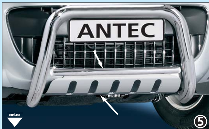
EU-horizontal pipe 35mm incl. under-ride protection plate (EU-certificate valid in combination with 12D4413 or 12D4713 only)
