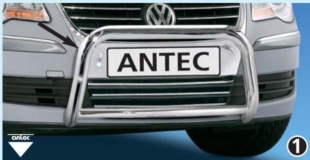
EU-pedestrian protection guard 60mm high with integrated horizontal pipe 42mm
