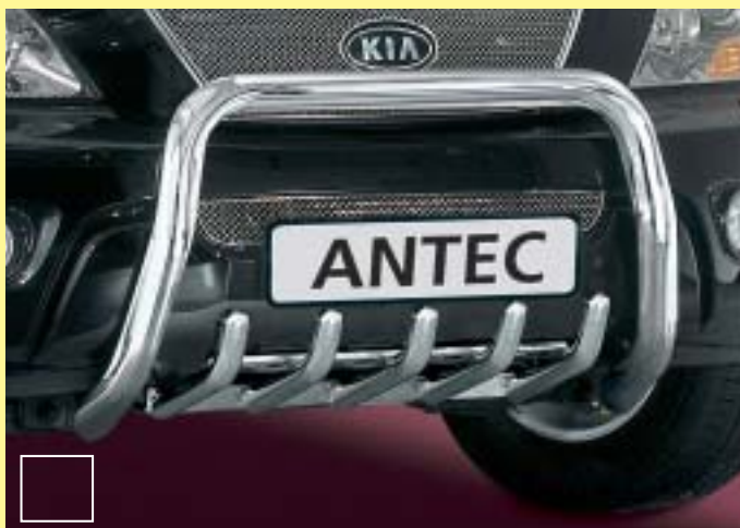
EU Pedestrian Protection Guard 60mm only mountable with 1714114 EU-pešacki zaštitni branik 60 mm EU-certificate is valid in combination with 1714114 only, Stainless steel/ Prohrom 171 4013
