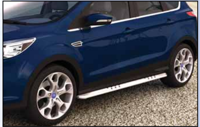
13L4351 Oval side bar 90 x 45 mm with dots Flankenschutzrohr 90 x 45 mm oval Stainless steel / Edelstahl
