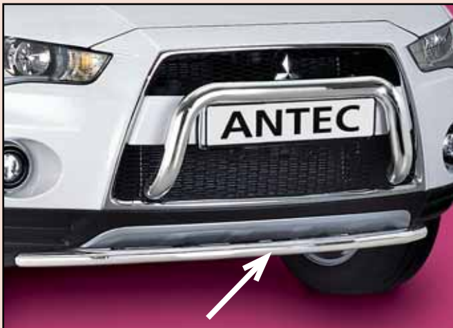
11Y4116 Spoilerbeskytter 42 mm rett Spoiler protective tube 42 mm straight Edelstål / Stainless steel
