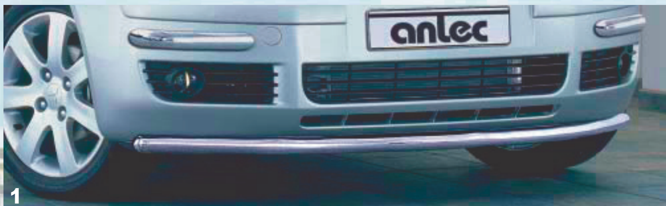
Spoiler protection pipe (straight) Spoilerbeskytter foran (rett) Stainless steel/Edelstål 189 4116
