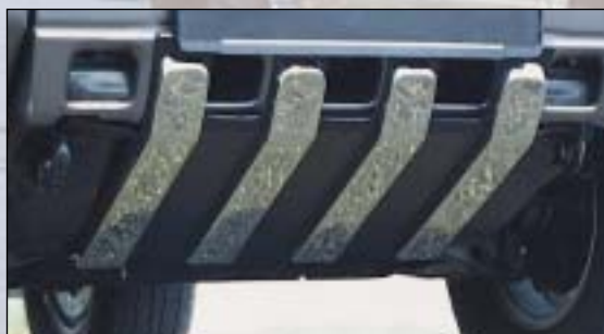
7 Front underride protection alleajoeste
