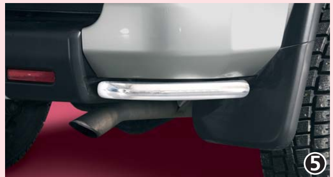
Bumper protection rear 42mm (compatible with tow-bar)
