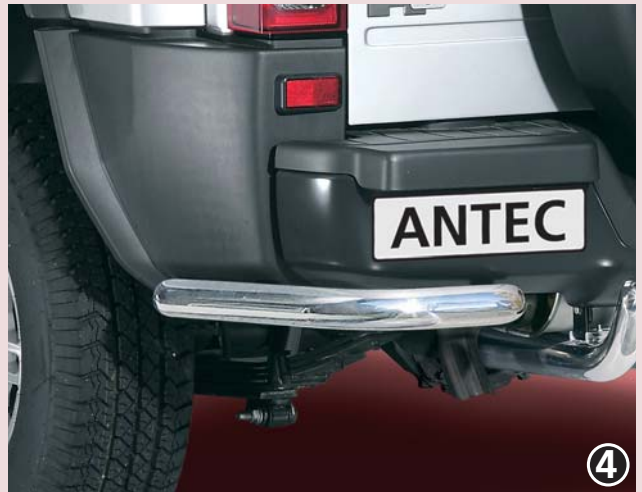
Rear bumper protection 60mm (TÜV-approval)
