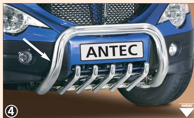
4 EU-pedestrian protection guard 70mm (EU-certificate valid in combination with 11L4014 or 11L4041 only) EU-ochranný rám 70 mm
