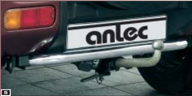
5 Rear bumper protector (Mountable with tow bar) Arka boru (Kombinierbar mit AHK) Stainless steel / Paslanmaz Çelik 102 4037
